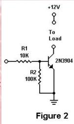
Finally, don't take the power from the GPIO pins, use a separate source - however, you will need to connect the GPIO ground to the buffer ground and, of course, the required GPIO control signal pin to the buffer input.
